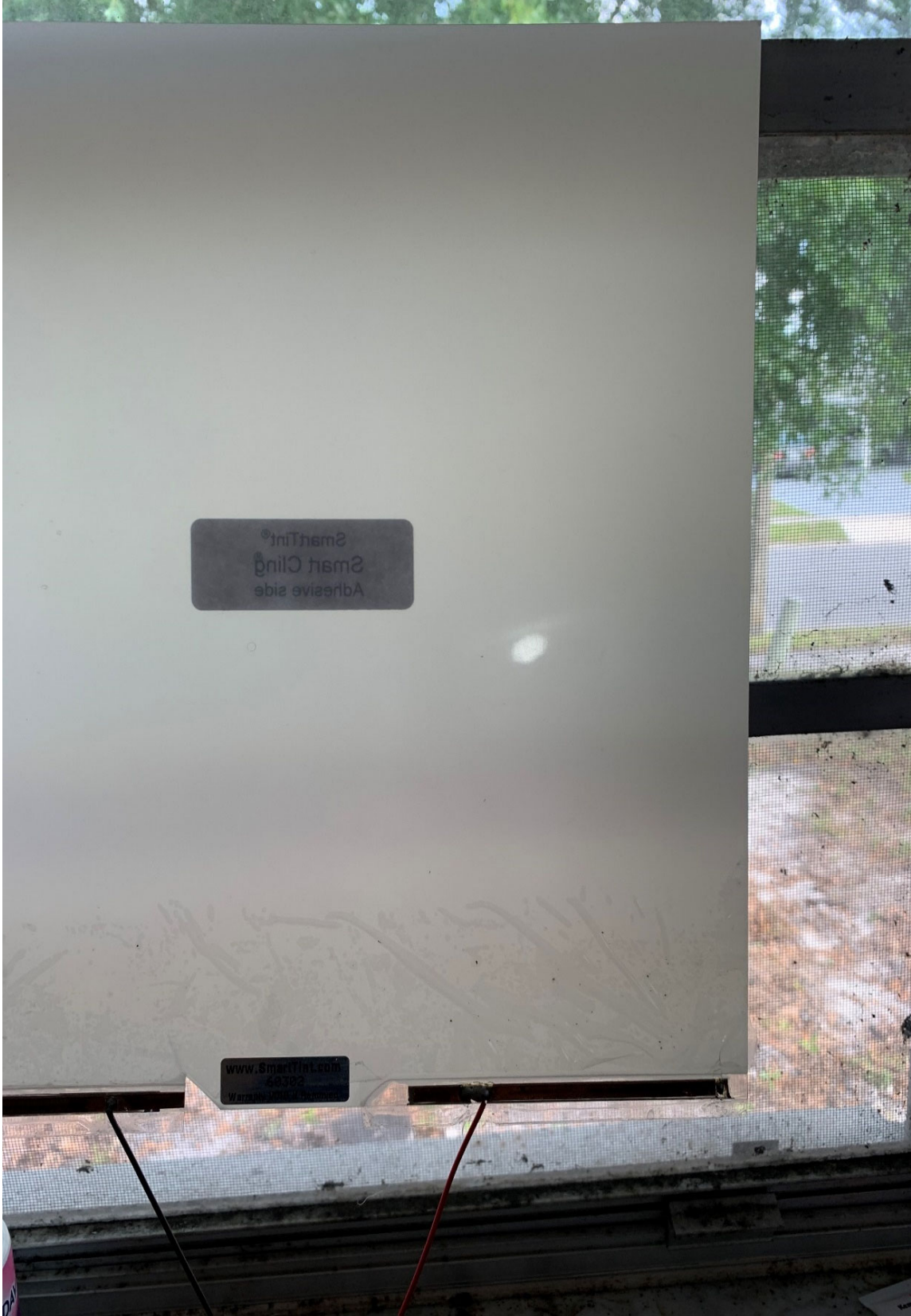
Figure 38: Smart Film (PDLC) in OFF state
