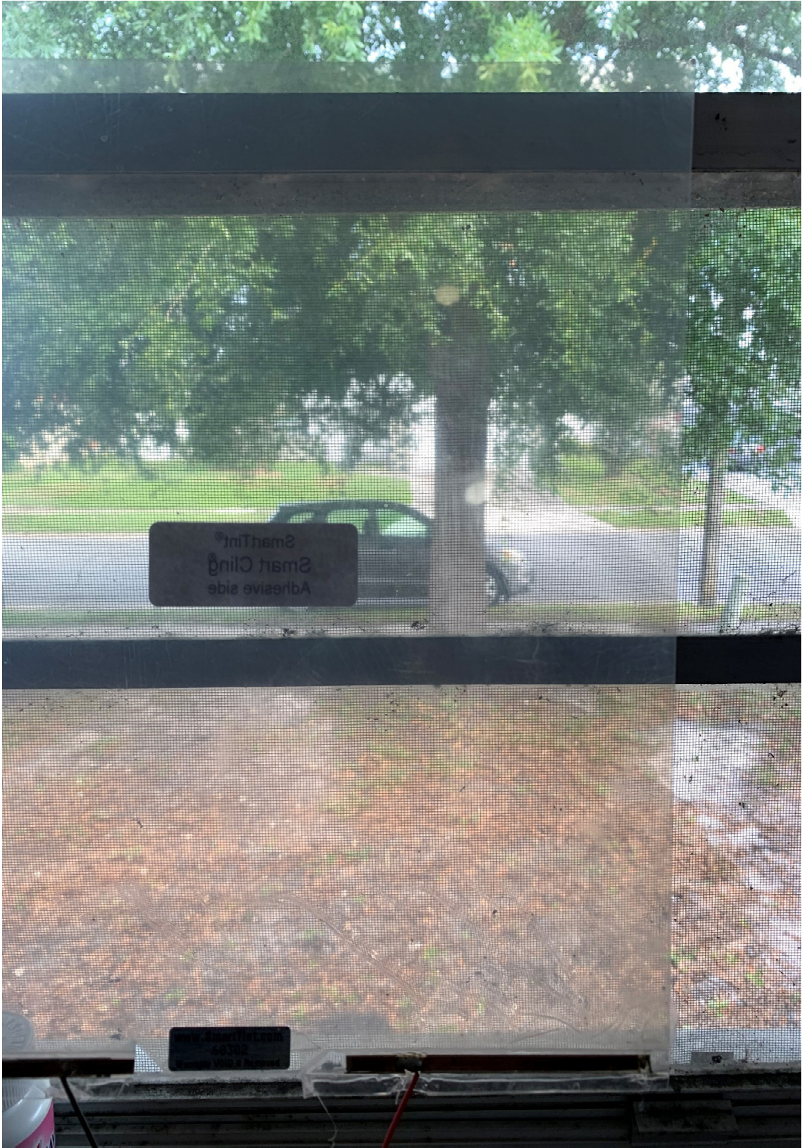
Figure 39: Smart Film (PDLC) in ON state
